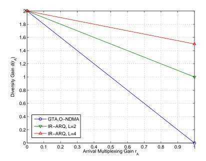
Fig. 6. Diversity gain versus the arrival multiplexing gain  $r_A$  for various two-user vector random access systems with random arrivals.
